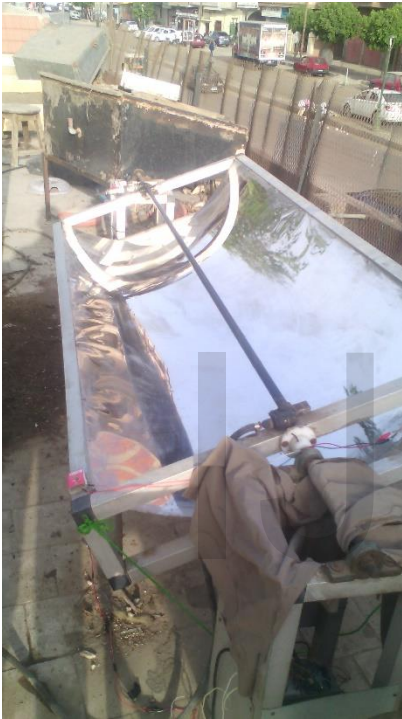
Fig (5). Photography picture of parabolic Trough without CO 2
